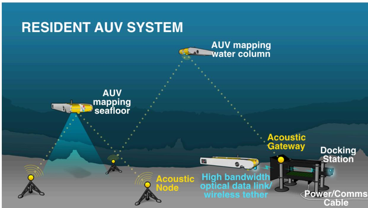
**Figure 1.** The overall concept and essential components needed for a R-AUV system. The power and communications chain starts at nodes connecting to land, and reaches one or more AUVs tasked with a wide range of potential missions. Such a system must incorporate real time or near-real time communications and the ability to recharge/refuel the vehicle, providing a means for routine or repeated operations, controllable from shore when necessary over deployment periods of months to years.
