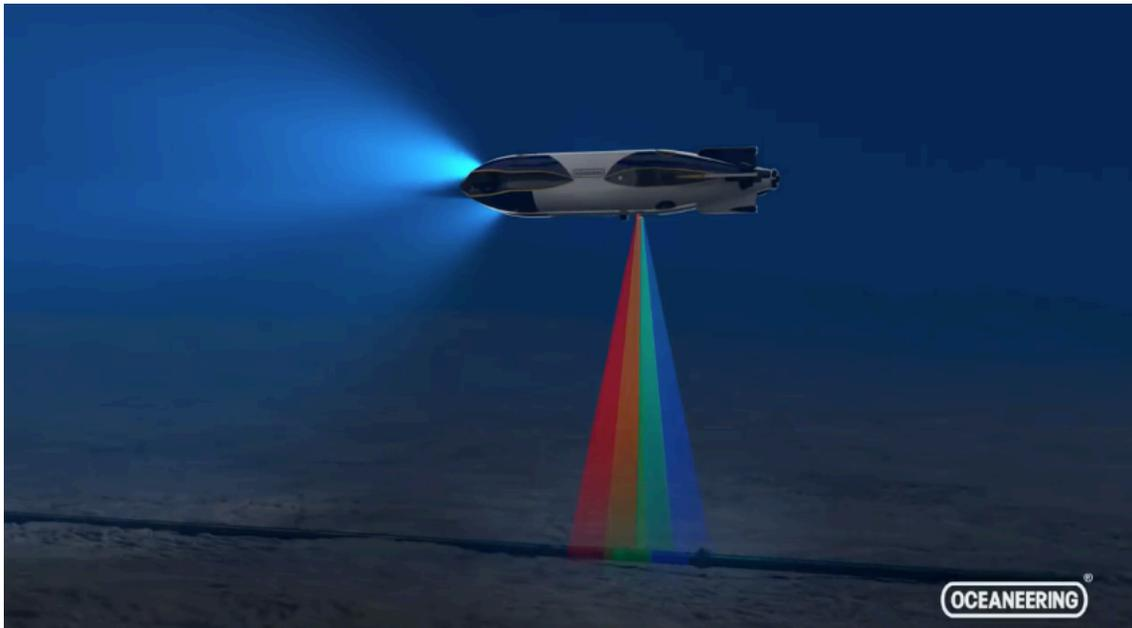
**Figure 10.** Conceptual art of Oceaneering Freedom vehicle performing autonomous inspection of a seafloor pipeline. (Image: Oceaneering)
