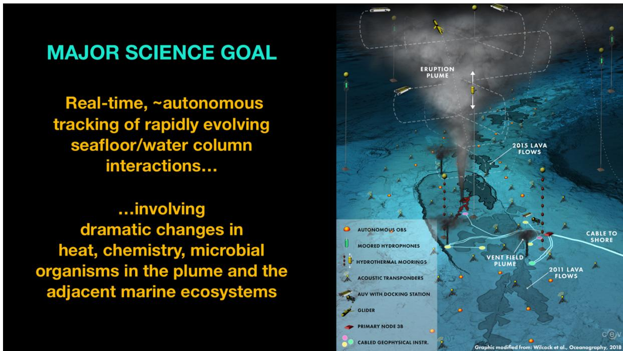
**Figure 5.** Artist's vision of the interactive examination of an eruptive plume at Axial Seamount. Conceptual rendering of an eruption on Axial Seamount with Sabertooth R-AUVs surveying the water column to define evolving dimensions, heat content, chemical and particulate load, and microbial signature of eruptive material, and its changing boundaries with the displaced pre-existing ambient oceanic ecosystems.
