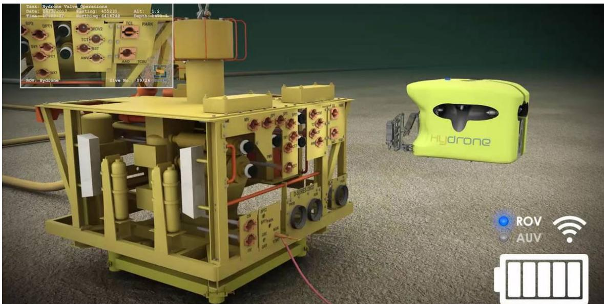
**Figure 11.** Conceptual rendering of Saipem Hydrone performing an autonomous, untethered intervention on a seafloor wellhead. (Image: Saipem)
