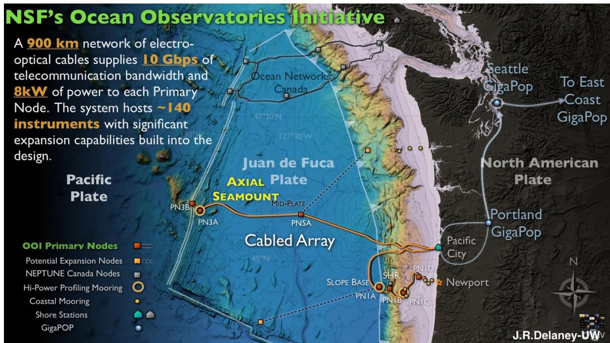
**Figure 2.** Stretching across the Juan de Fuca tectonic plate, the OOI-CA is a 900-km network of electro-optical cables that supplies up to 10 Gb/s bandwidth and as much as 8 kW of power to each of six primary nodes (red squares). At present (2019) the system hosts more than 148 instruments; the cabled array was designed to support significant expansion potential and could host a R-AUV docking station.
