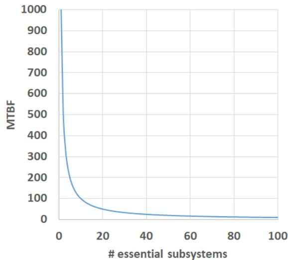
**Figure 13.** Generic plot of reduction in system mean time between failure (MTBF) as the number of essential subsystems increases.
