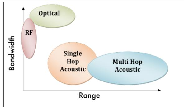
**Figure 12.** Relative range (distance spanned) vs. bandwidth (amount of data transferred) for subsea wireless options.
