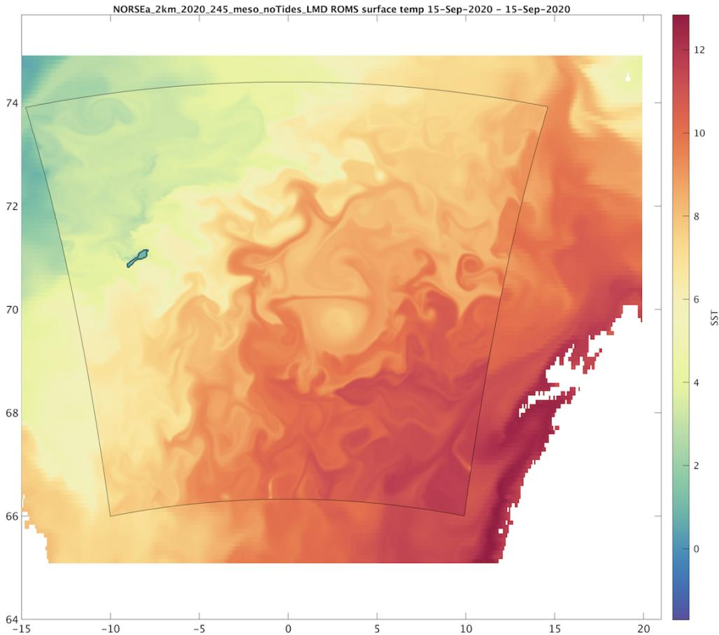
**Figure 7.** Example hindcast simulation of the Nordic Seas. The outer region is the GLORYS12V1 Mercator Ocean Model simulation GLOBAL\_REANALYSIS\_PHY\_001\_030 and the inset is a nested 2-km simulation using the ROMS ocean modeling system.
