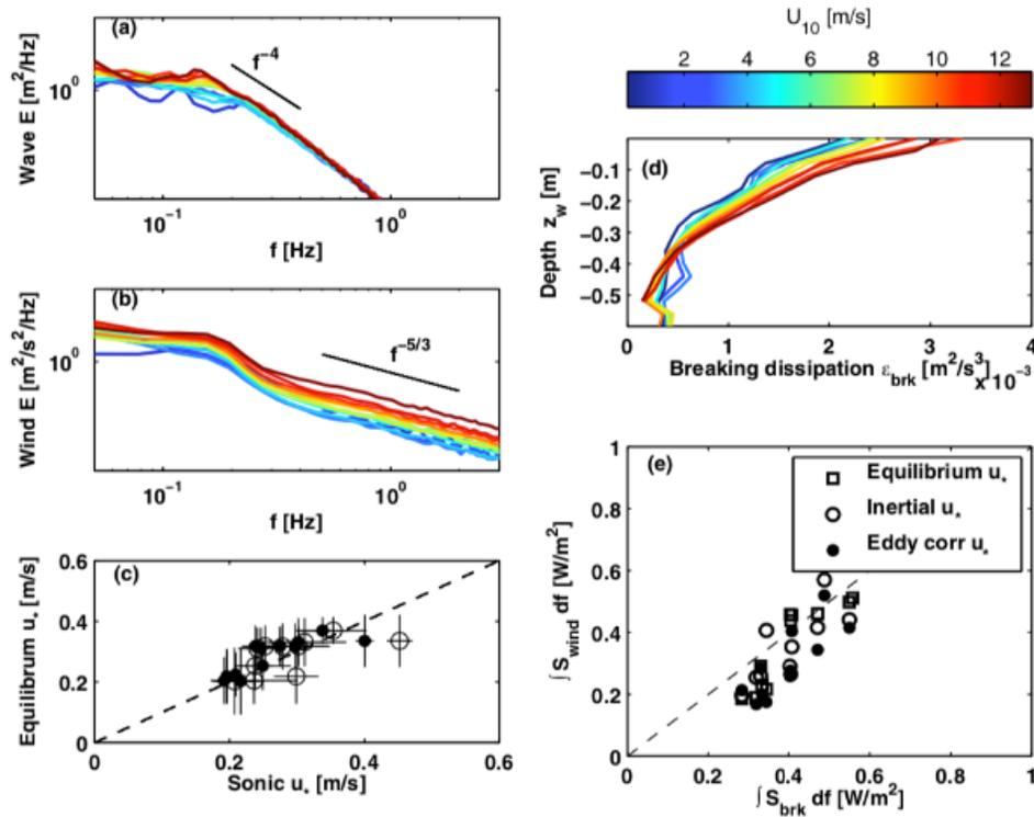
**Figure 3.** Example of wind–wave equilibrium over a range of conditions observed with SWIFT buoys: (a) wave spectra, (b) wind spectra, (c) wind friction velocity, (d) profiles of turbulent dissipation rate in the ocean surface layer, and (e) balance of wind input TKE flux with dissipation in the water. Reproduced from *Thomson et al. (2013)*.
