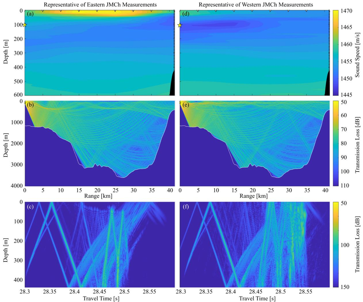
**Figure 6.** (a) Sound speed profiles constructed from CTD measurements shown in Fig. 7(c, f) from *Wang et al.* (2021) with the location of the acoustic source at 0 km to the location of the acoustic receiver array at 42 km. (b) Transmission loss for a 1-kHz source at a depth of 100 m. (c) Impulse response for measured by a vertical line array for a 1-kHz bandwidth centered at 1 kHz. (d–f) same as (a–c) except using CTD measurements shown in Fig. 7(d, g) from *Wang et al.* (2021).
