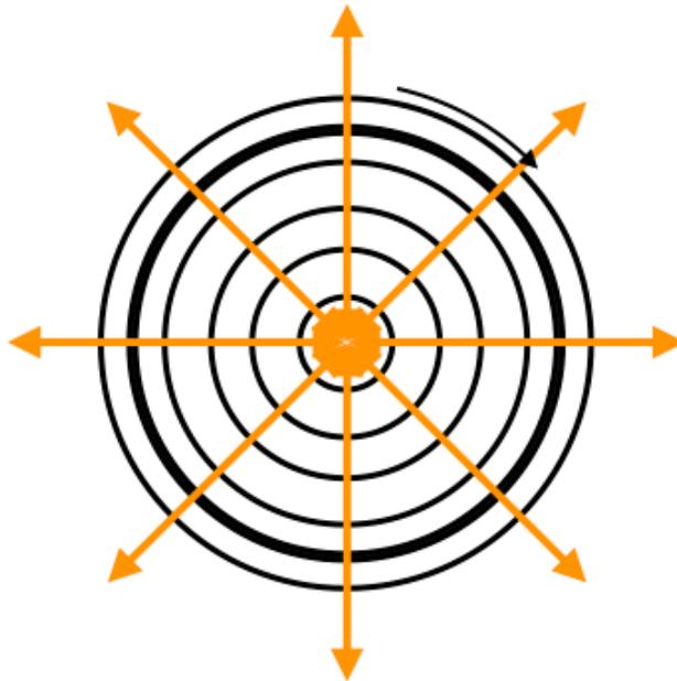
**Figure 5.** *Glider survey of an eddy. Gliders transit radial lines (orange arrows) in a mesoscale eddy while it propagates to the west.*
