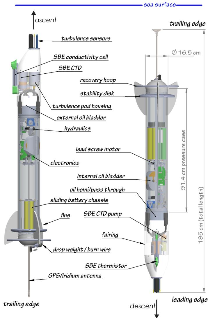
Figure 12. Schematic of Flippin'  $\chi$ SOLO float.
