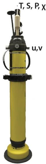
**Figure 11.** Profiling EM-APEX floats are equipped with a sensor package to measure 2–3 m temperature and salinity with ~ 5 m horizontal velocity, and 1 m microscale temperature variance dissipation rate to a maximum depth of 2000 m. Velocity is inferred from the electric field induced by ocean currents moving through Earth’s magnetic field, resulting in a voltage drop across the insulated float body. Microscale temperature is measured with a pair of Rockland Scientific fast thermistors.
