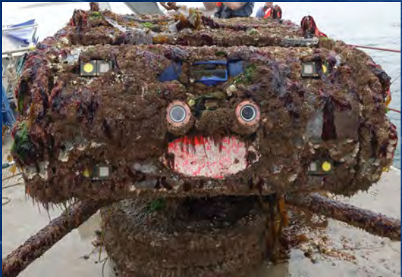
The AMP following a 118-day deployment (96% system availability) in Sequim Bay
