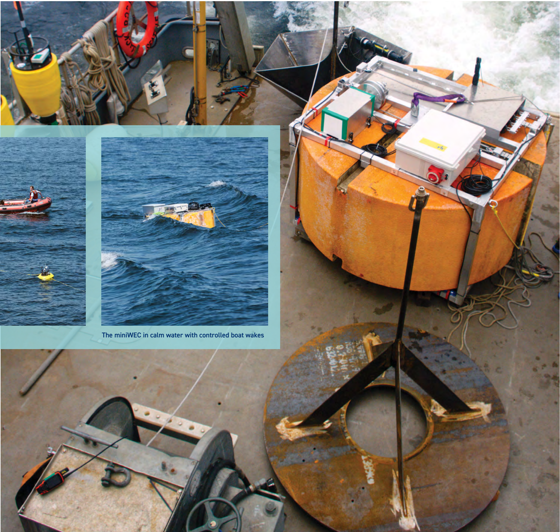
The miniWEC on the deck of R/V Robertson during tests of flat and conic heave plates
