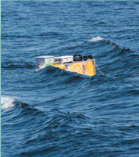
The miniWEC in calm water with controlled boat wakes
