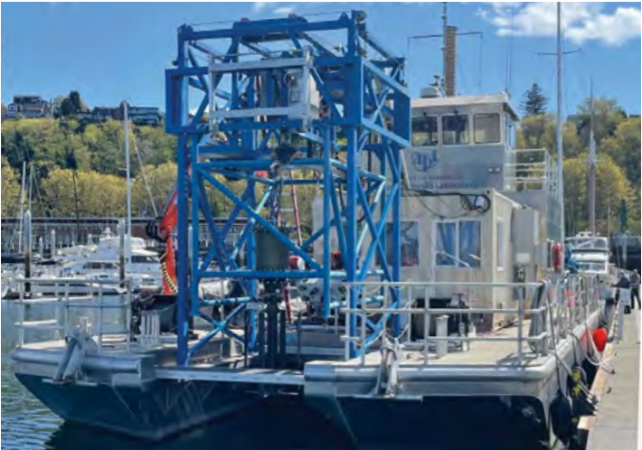
The Turbine-Lander rotor (and VAMP) mounted on R/V Light prior to its deployment in Agate Pass.
