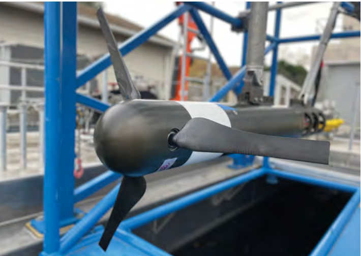
Axial-flow turbine installed on R/V Light for testing under propulsion. The rotor is approximately 1 m in diameter and the unit is equipped with multiple 6-axis load cells to measure loads and system performance.
