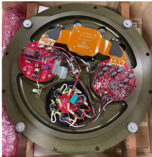
Figure 9: MPC on the PTO housing endcap with the load dump (near the bottom).
