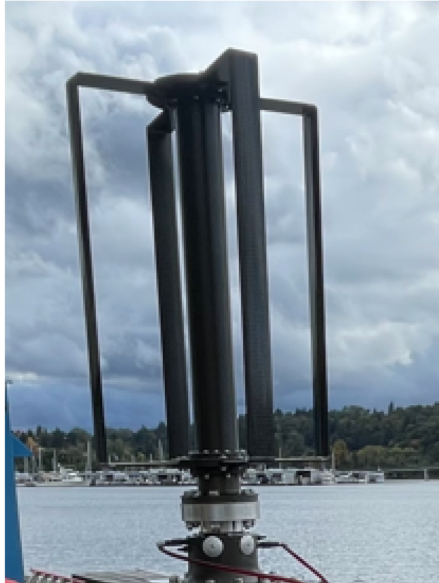
Figure 3: The 1st generator rotor installed on the Turbine Lander prior to deployment in October 2023.
